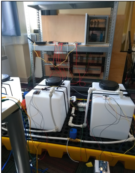
Photo of the testbed showing water tanks and control systems in the background
